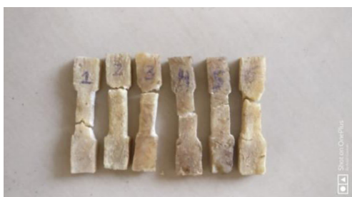
Fig.8 Specimen after tensile test
