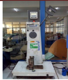
Fig.3. Charpy Impact Test
